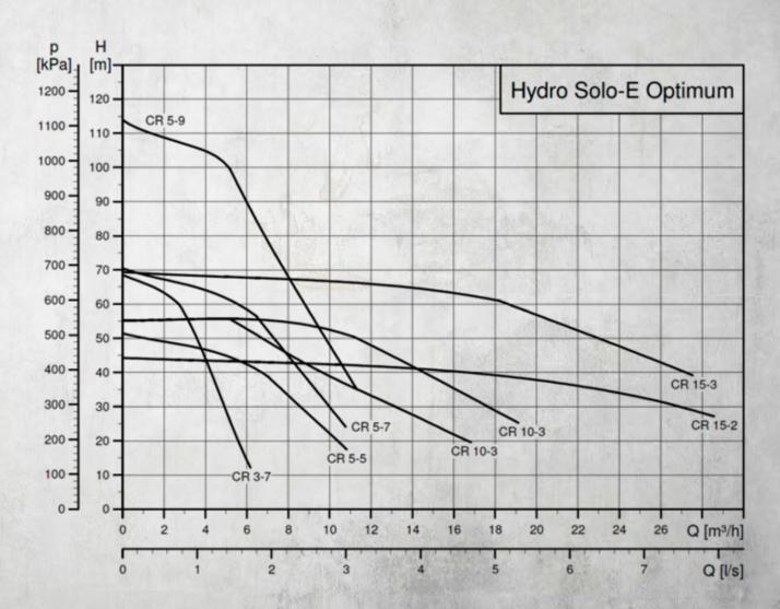
When the load of the motor reaches maximum, the motor derates in speed to keep the power constant.
