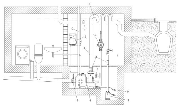
Fig. 1 Installation example of a MULTILIFT lifting station
