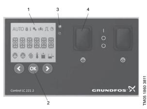
Fig. 40 Control panel of two-pump controllers
