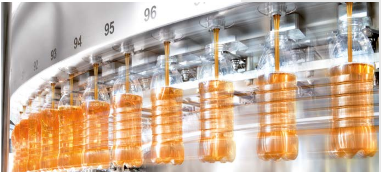
The high accuracy and performance of these filling machines is achieved through the use of magnetic flow meters managed by a high speed processor for flowrate control in real time.
