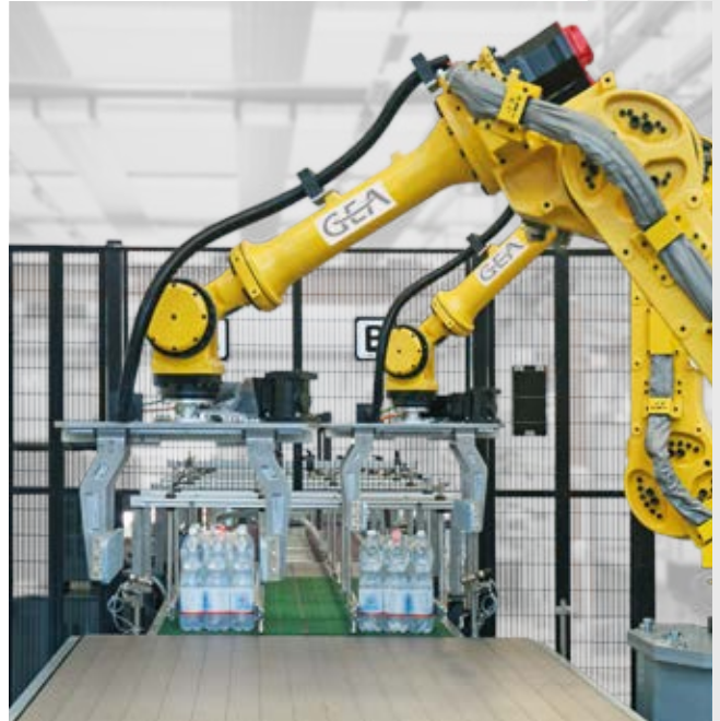
The layer preparation system Polaris F can prepare an entire layer of products (even particularly unstable ones) without any jolts during the repositioning phases.
