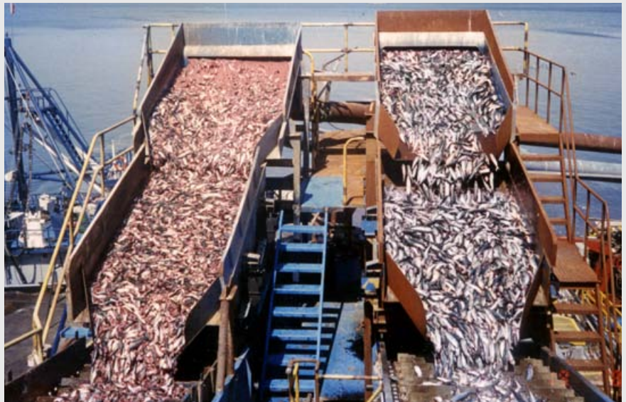
Landing fish: considerable reduction of rejects and lower pollution with blood water when pumping with progressing cavity pumps (right) instead of centrifugal ones (left).
