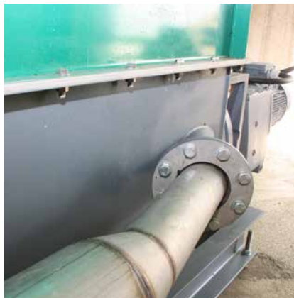
For improved substrate mixing the supply of the liquid is opposite to the direction of pumping.
