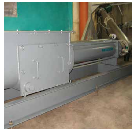
Easy maintenance through large inspection cover.
